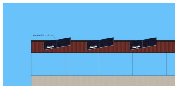
Figure 14 Suitable position of PV Panel
